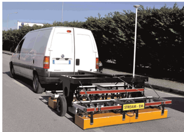
Figure 3. The latest development in multichannel, multifrequency antenna systems with different polarizations: the 40 channel system called Stream EM from Ingegneria dei Sistemi, S.p.a. (IDS) (courtesy of IDS). This figure is available in colour online at www.interscience.wiley.com/journal/arp
