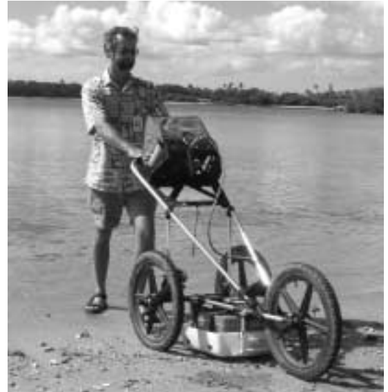
Figure 2. The GSSI SIR-3000 system with survey wheel, 400 MHz antenna and control unit with flash memory chips for data storage and playback.
