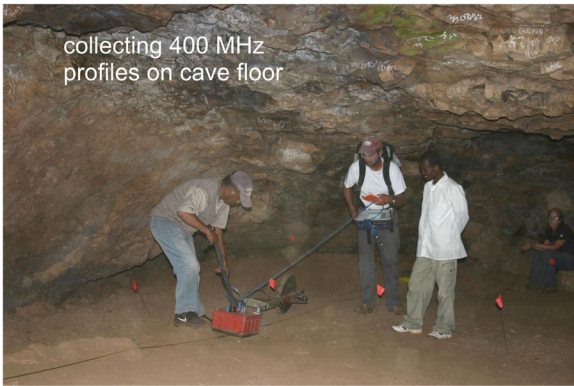
Fig. 20 Collecting 400-MHz GPR profiles at Tuwatey Cave
