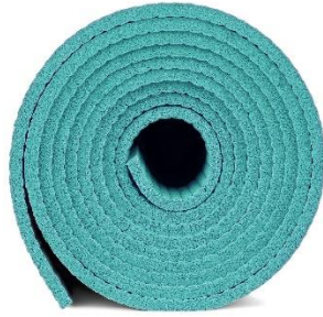
Figure 10: PVC yoga mat 1/4 inch thick (8 mm) used to cover the sand
