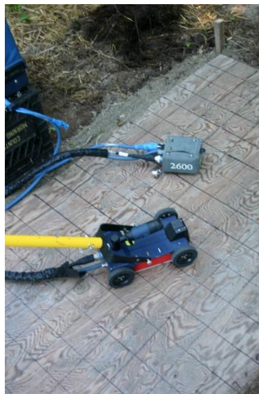
Figure 6: The 2.6 GHz antenna used on the plywood surface.
