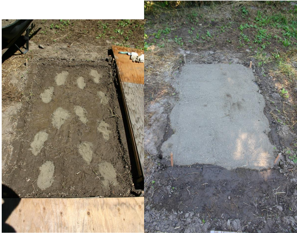
Figure 9: Covering the model with basalt sand
