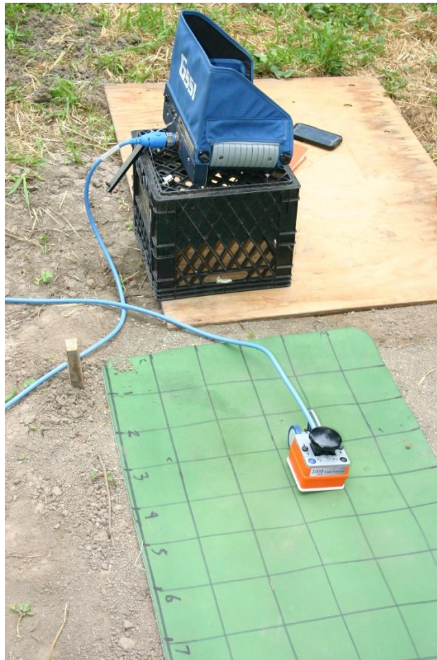
Figure 11: Yoga mat that was gridded in the same way as the plywood surface. This mat filled in the minor undulations in the sand surface, removing any air pockets that were present. The antenna here is the 2 GHz palm antenna.
