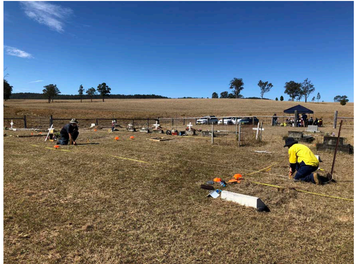
At Baryulgil Aboriginal Cemetery NSW multiple GPR grids were established to avoid the surface gravestones, fences and ornaments, typical of historic cemeteries (Source: E. St Pierre).
