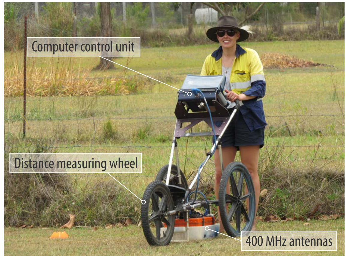
Ground-penetrating radar system, this one is a GSSI SIR-3000 system with 400 MHz antennas mounted on the “baby jogger” cart being used at Coraki Cemetery, on Bandjalang country, NSW (Source: Virtus Heritage).
