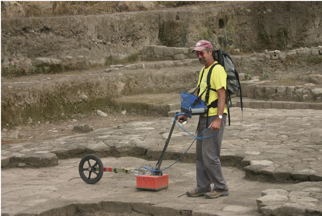
Figure 1. GPR equipment including 400 MHz transmission and reception antennas in the fiberglass box, attached survey wheel for distance measurement, and the radar control unit and computer attached to the operator's back. This is a Geophysical Survey Systems SIR-3000 system.
